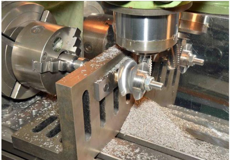
Above. Photo 2: The flared top surface of the chimney base was machined using a  $\frac{3}{4}$ in. HSS ripper cutter.
